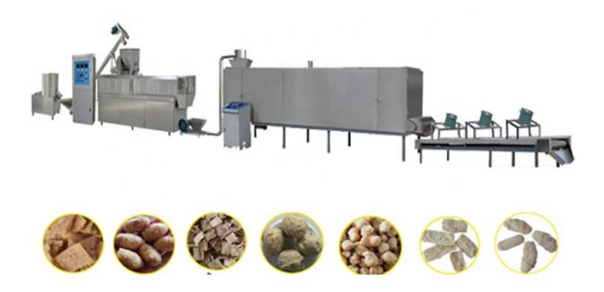
The fully automated production method requires close coordination of all equipment, which will provide us with very high production efficiency and production quality. The advanced extrusion technology not only retains most of the nutrients in the raw material, but also allows the production of a mellow tasting bean meat that tastes very similar to meat
