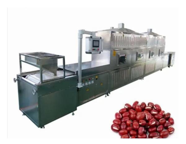
In the **Industrial Microwave Food Proce** process, the microwave equipment can quickly heat food, and microwaves can be turned into heat in seconds. Microwave equipment has the characteristics of selective heating, can be more evenly heated food. Because the microwave is easily absorbed by the material containing water, so there is little waste. In addition, the microwave also has the role of sterilization, which can well protect the nutrients in the food.
