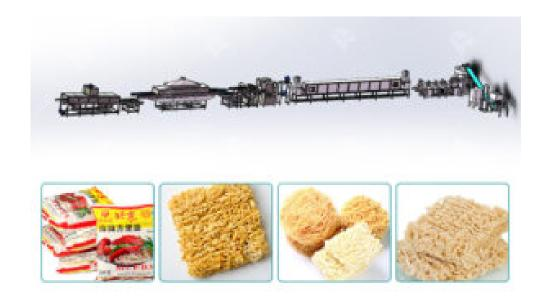
Packaging material preparation: This step includes cleaning and sanitizing packaging materials, such as dough bags or cups, and doing some special processing, such as printing and cutting. Instant noodle manufacturing: Mix the prepared noodles with seasonings, and process them by steaming or hot air drying, and finally form the finished instant noodles.
