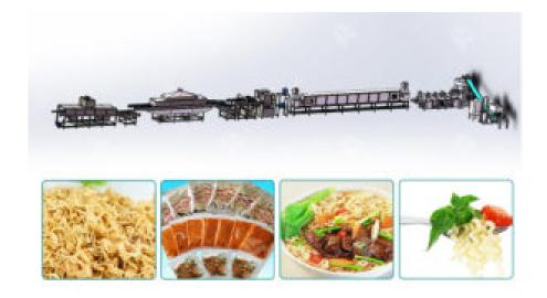
Noodle production: mix flour and other raw materials with an appropriate amount of water through a mixer to form batter, and then make the batter into noodles through gelatinization, hot air steam and other processing technologies.
