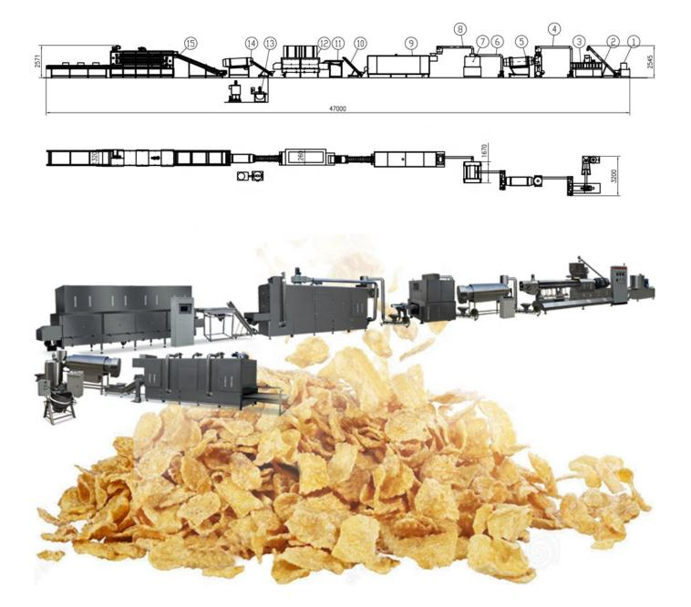
At this point, the corn flakes are basically formed, and then the corn flakes are transported into the oven for hightemperature baking, so that the corn flakes lose moisture, which can make the corn flakes more crispy, and can effectively extend the shelf life, baking temperature and time Adjustable.
