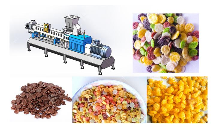
The whole corn flakes production line can automatically complete the production from mixer, screw conveyor, twin screw extruder, cooling conveyor, air conveyor, flaking machine, air conveyor, pre-dryer, hoister, vibrate feeder, baking machine, sugar sprayer, vibrate feeder, multi-layer oven and cooling conveyor to the finished product.
