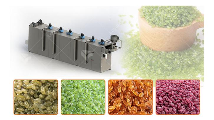
The whole nutrition rice production line can automatically complete the production from mixer, screw conveyor, twin screw extruder, vibrate cooler, air conveyor, multi-layer dryer and cooling conveyor to the finished product.
