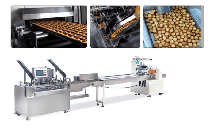
BISCUIT SANDWICHING MACHINE FOR SALES We provide--- the most reasonable, economical and stable design biscuit sandwiching machine. Saving money and time for the client. SANDWICHING BISCUIT PRODUCTION LINE FOR A BISCUIT FACTORY Flour Mixer-Roll Cut Biscuit Form Machine-Tunnel Oven-Oil Sprayer Net Belt Cooling Conveyor -Electrical Control Box -Automatic 2+1 Biscuit Sandwiching Machine--Packing
