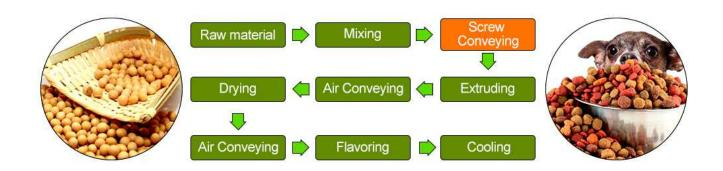
Raw material---Mixing---Screw Conveying---Extruding---Air Conveying---Drying---Air Conveying---Flavoring---Cooling
