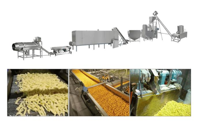
Mixer→ Screw conveyor → Rotary head extruder → Hoister → Separate drum → Air conveyor→ Dryer → Flavoring machine
