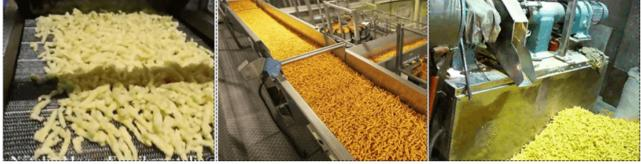
Mixer → Screw conveyor → Rotary head extruder → Hoister → Separate drum → Air conveyor → Dryer → Flavoring machine
