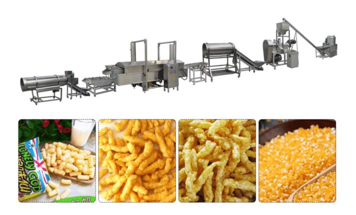
Mixing Machine →Screw Conveyor →Rotary Head Extruder →Hoister →Separating Drum →Hoister →Continuous Fryer →Vibrate De-oil Machine →Flavoring Line
