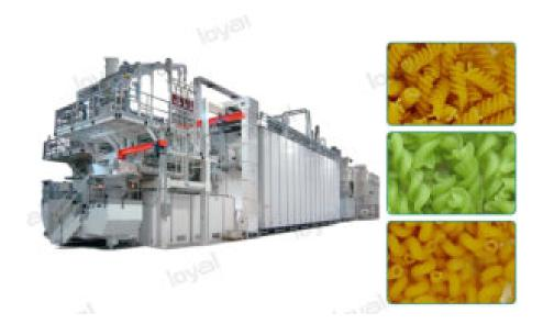
This machine uses corn starch and potato starch as the main raw materials, and uses a unique extrusion molding process to achieve a good sensory effect in the shape of the product. The production line has reasonable design, strong stability and high degree of automation. The main engine adopts advanced frequency conversion speed regulation technology, which is highly efficient and energy-saving. Precise parameter control and good process flow ensure stable quality of processed products.
