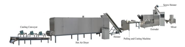
Automatic Macaroni Pasta Production Line is absorbing the advanced foreign technology based on research and development performance and technical quality indexesreach the international advanced level of the similar equipment. This production line from the raw material ingredients, raw material, conveying, extrusion, baking until acomplete product. Can produce all types of pasta, spaghetti food.
