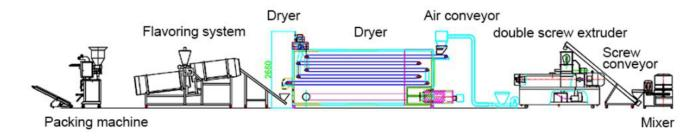
This line has with Mixing system, with Extrusion system, with Drying system, with Flavoring system, with Packing system.
