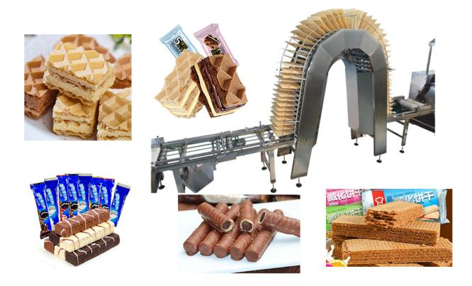
Wafer sheet baking of Wafer Making Machine from oven, automatically transfer to cooling tower and cooling in the air. Cream will be automatically applied on wafer sheet, after the cooling from cooling cabinet, wafer book cut on cutting machine.
