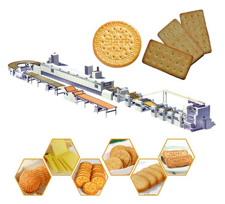
The baked biscuits are transported to fuel injection machine. And through the conveyor. After the fuel injection, the color, fragrance. Then taste of the biscuits are more distinctive. It can effectively improve the quality of the biscuits. Afterwards, the biscuits cool by the cooling machine. That step is to ensure that the biscuits packag. The quality of the product and effectively extend the shelf life. And finally use the packaging machine for packaging. So that the production is completed.
